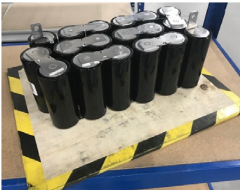
Figure 1. Example of good handling of the cell-pack. The cell-pack is placed on a flat structure which supports all the cells.
