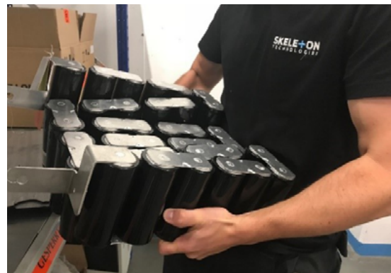
Figure 2. Example of not allowed method of handling the pack. From the image it can be seen that the cell-pack is deformed, this type of deformation can cause cell damage.
