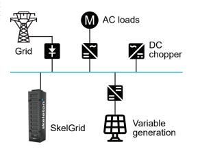
Skelgrid directly connected to DC bus systems or VSD DC link
