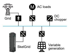
Skelgrid connected to DC bus systems through DCDC converter
