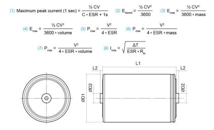
(9) The stated maximum peak current should not be exceeded during use. If the limit is to be exceeded by the customer, Skeleton must be consulted beforehand and give approval for the exceeded power load. Typical value represents the mean production sample value. Rated value represents the absolute minimum capacitance or maximum ESR value of production sample.
